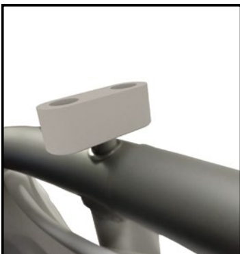
8. To install the optional lights, place the lighting clip into the top hole of the frame.
