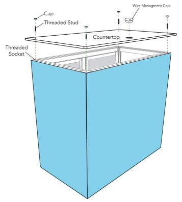
7. Install the countertop using 4 threaded studs and 4 caps. Optionally, install the wire management cap over the wire management port.
