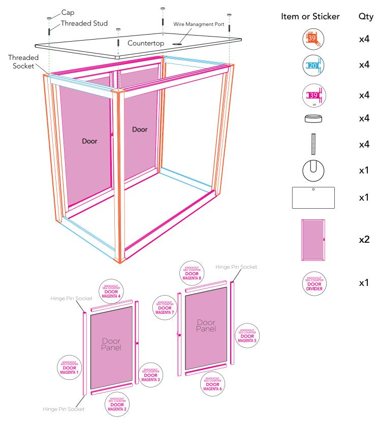
1. Assemble the doors, trapping the door panels inside. Note: Doors may already be preassembled.
