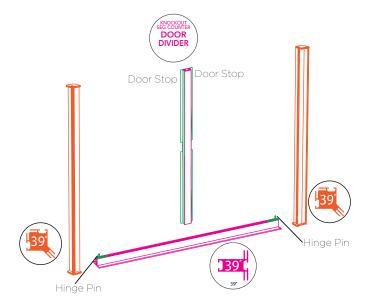
2. Assemble the counter side that will hold the two doors. Attach the door divider in the center of one of the 39" pieces with two hinge pins. Note: The door stops will be on the side facing the inside of the counter.
