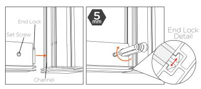
When attaching two pieces together, slide the end lock inside the channel of the other piece. Tighten the set screw to cause the end lock's jaws to spread and grip the inside of the channel. Do not overtighten.
