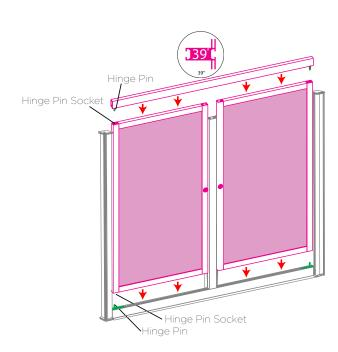
3. Complete the counter side by installing the doors. The hinge pins slide inside the hinge pin sockets on the door vertical. Hold the doors in place while installing the top bar with hinge pins.
