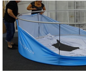
7. Begin pulling the graphic up the frame. Make sure the grommets in the graphics line up with the black circular "button" on top of the frame.
