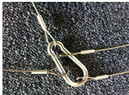
10. Connect other ends of wires to caribeenner and hang the display up.
