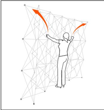
1. Expand the frames so they stand upright with the adjustable feet on the floor.
