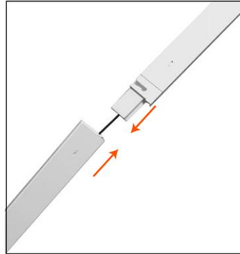
3. Assemble the channel bars. Slide the channel bar's end hook into the slot in the corner hub. See diagrams at the bottom of this page for channel bar locations.
